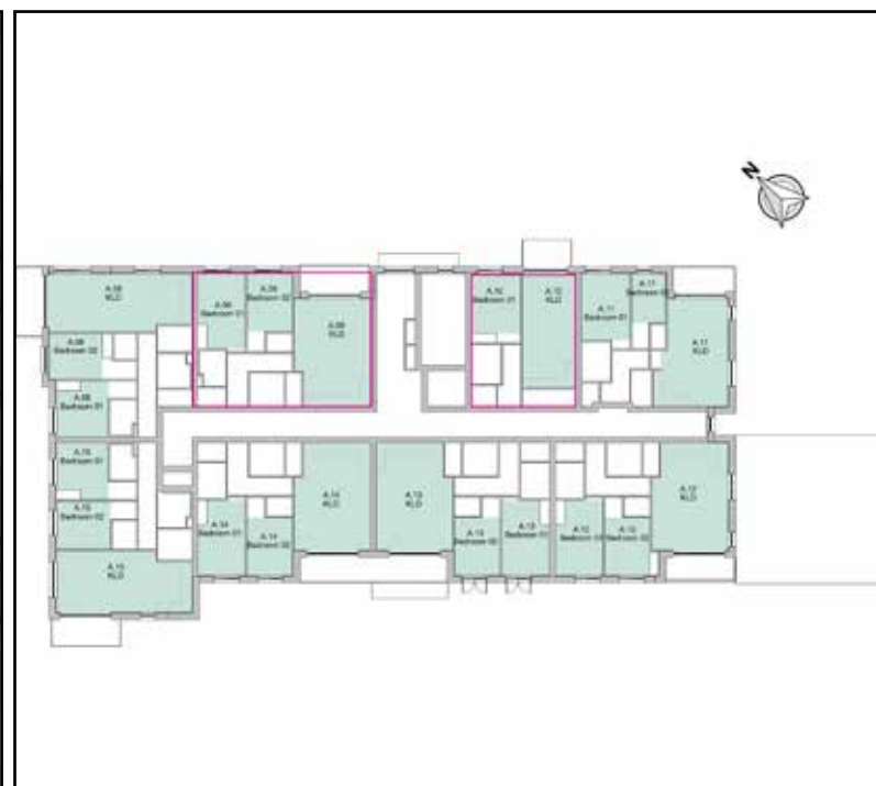
Figure 3.11: Underperforming single-aspect units highlighted
